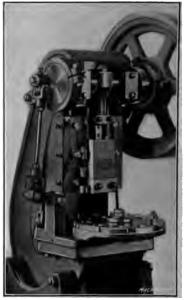
Fig. 8. Ratchet Dial or Rotating Feed Mechanism
